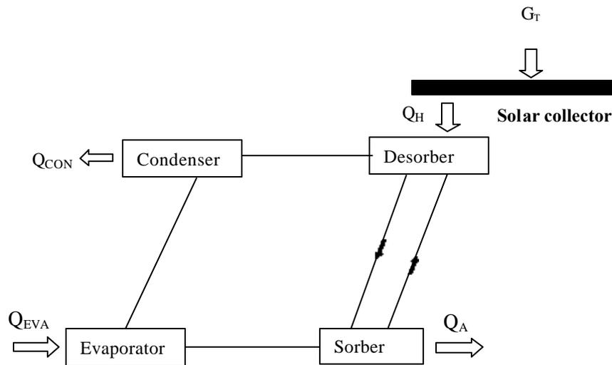
Fig.1 Schematic of a solar driven sorption refrigeration system
