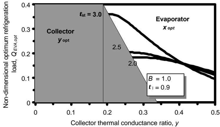
Fig.2 Effects of collector stagnation temperature on refrigeration load
