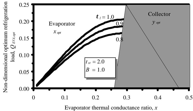
Fig.4 Effects of non-dimensional refrigeration space temperature on refrigeration load
