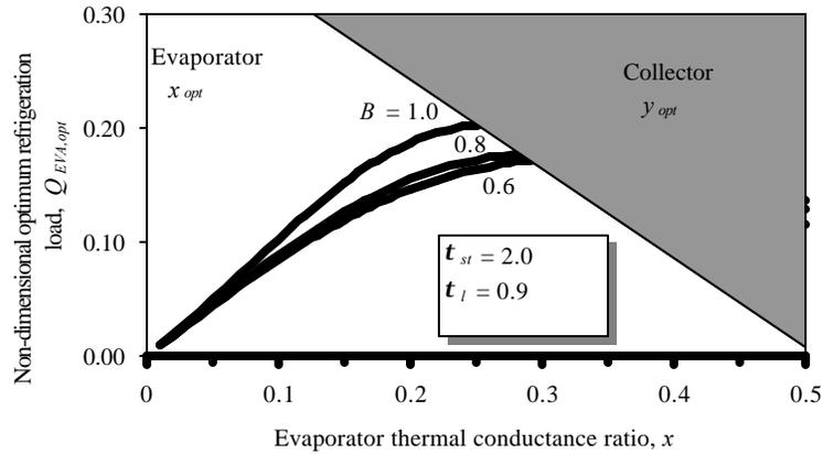
Fig.3 Effects of non-dimensional collector size on refrigeration load
